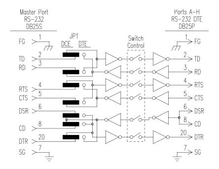
Figure 5. Simplified RS-232 Schematic
